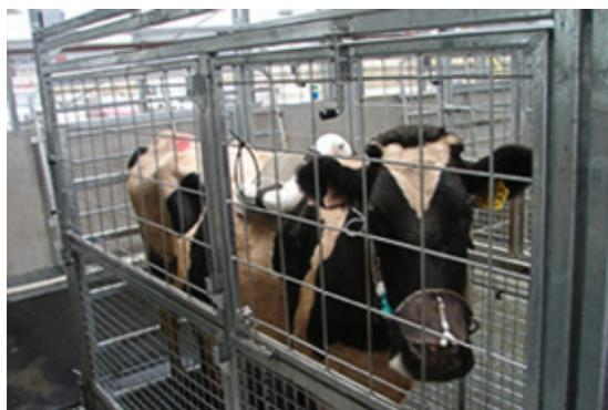
Dairy cattle fitted with  $\text{SF}_6$  apparatus for Methane measurements
