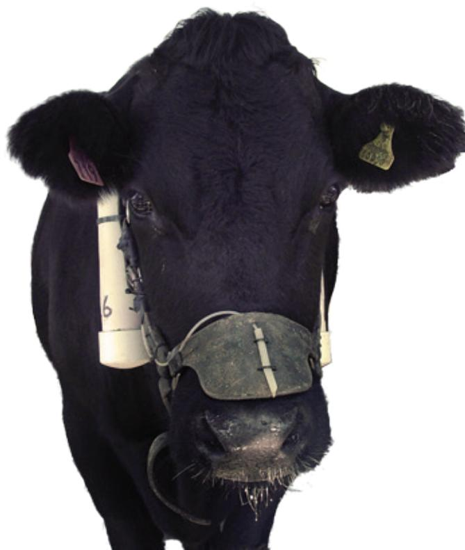
Cattle wearing neck harness for measuring CH<sub>4</sub> at grazing using the SF<sub>6</sub> technique
