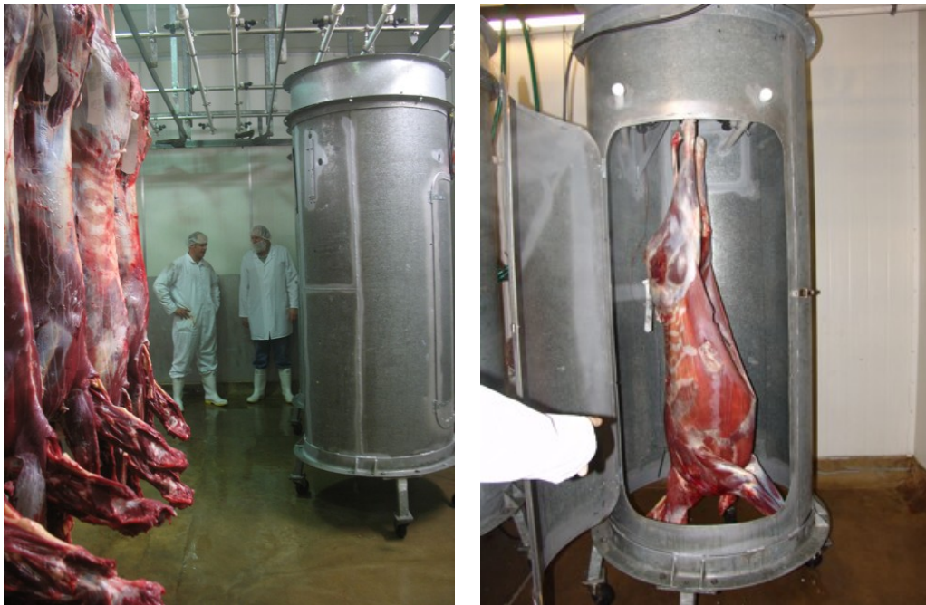
Figure 1. Spray chilling silos in place in the chiller at Silver Fern Farms deer slaughter premises in Rotorua.
